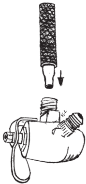
Installation of Fuel Shut Off & Gas Tank Screen (A9193T) into A9189A
